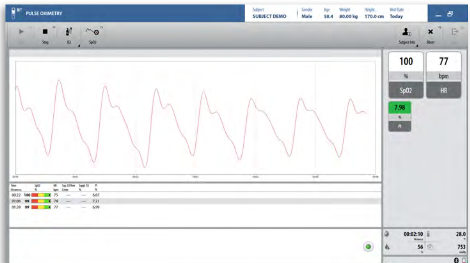
Pulse oximetry spot check real time interface with plethysmographic curve and Perfusion Index monitoring.
